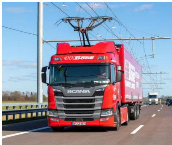
Fig.1 Image of a truck driving on the E highway using overhead lines
